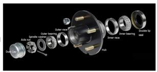
No parts are more critical for the dependable performance of your trailer than the bearings, races, and seals. To ensure that your trailer performs reliably, you should inspect the bearings, races, and seals and repack the bearings every 12 months.
