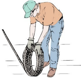
Correct ways to unreel and uncoil wire rope.
